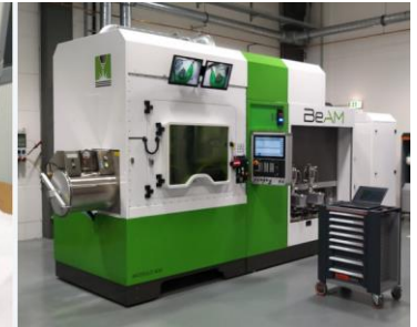
DED unit at MTA
